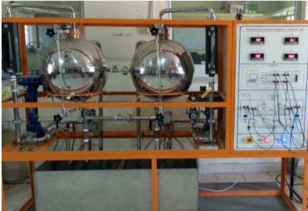
Figure. 5: Real time setup of coupled Spherical tank system
